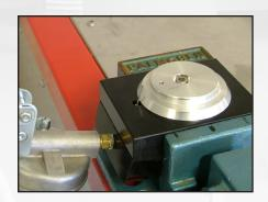
2. Install appropriate bearing seat onto the packer base. Bearing seat is aligned with a locating dowel.
