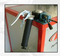
1. Place bearing packer in standard bench vise. Install grease cartridge and bleed grease gun. (Instructions included separately.)
