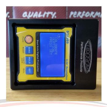
• Final step, rotate the gauge 180° and press SET. Once you have done this last step, the gauge has been fully calibrated and ready for use.
