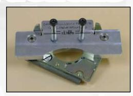
2. Attach caliper mount to jig using the screws provided. Adjust the locating pins to the disc diameter desired. Caliper mount bolts to the back side of the jig, opposite the engraving and locating pins.
