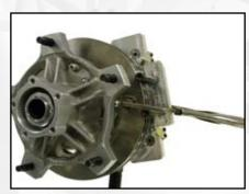
3. Place the jig face onto the brake disc. Allow the locating pins to touch the outer diameter of the disc. Using a pair of vise grips or a C-clamp, clamp the jig to the disc. You may add a second clamp to the disc to prevent the hub from spinning.
