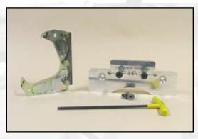
1. Prepare caliper mount and spindle for installation. Mount the hub and brake disc onto the spindle.
