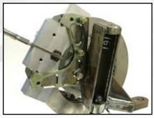
4. Weld the caliper mount or mounting tabs to the spindle body. Weld small stitches on opposite sides to prevent pulling. Remove the hub and disc to complete welding.
