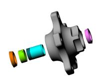
**Step 1:** With bearings clean and dry (no grease), adjust bearing spacer out to 3/4 of it's maximum length.
